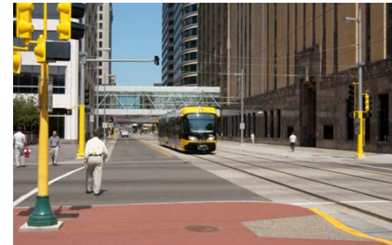
Example of Light Rail on Embedded Track
