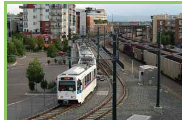
LRVs can navigate tight turns and accelerate and decelerate more quickly than vehicles like Diesel Multiple Units and Amtrak trains.
