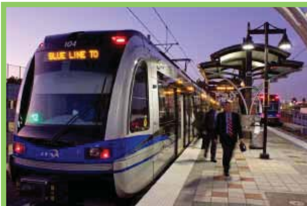
Light Rail Vehicles (LRVs) are electrically powered vehicles and operate on their own tracks, in a dedicated right-of-way.
