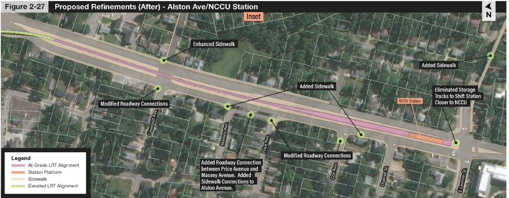
Figure 2-27: Illustration of Proposed Refinements – Alston Avenue/NCCU Station Inset
