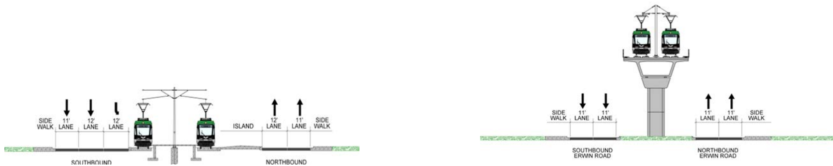
Figure 2-21: Cross Sections – Duke/VA Medical Centers Station (Previous Design at Left; Proposed Refinements at Right)
