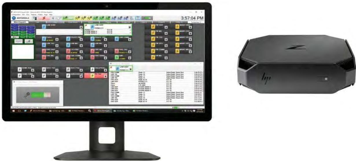
Figure 2-1: MCC 7500E Dispatch Position provides a small form factor, familiar GUI, and advanced features.
