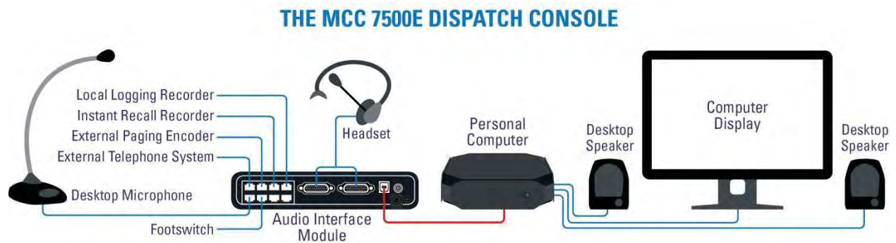
Figure 2-3: MCC 7500E Dispatch Position supports multiple accessories.
